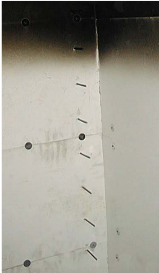
Figure 2.5. The sidewall thermocouples in the adjacent compartment.
