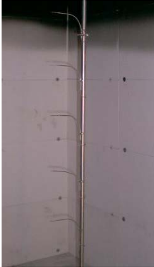
Figure 2.4. Example of a thermocouple tree.
