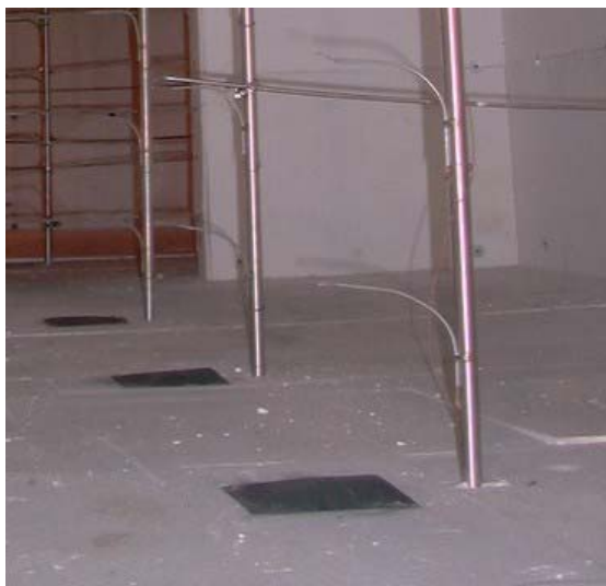
Figure 2.8. The floor thermocouple plates in the adjacent compartment.
