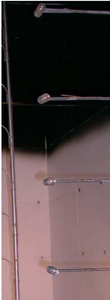
Figure 2.12. Bi-directional probes in the front opening of the compartment.
