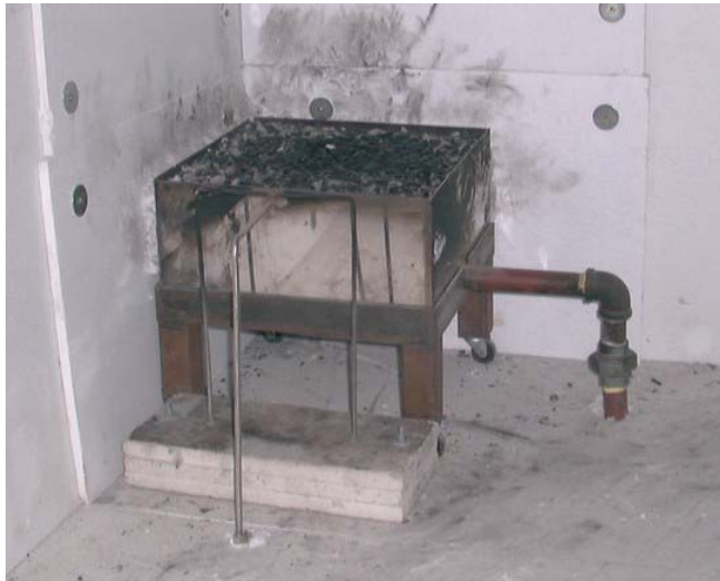
Figure 2.3. The burner in the corner location, with spark igniter and pilot flame in foreground.
