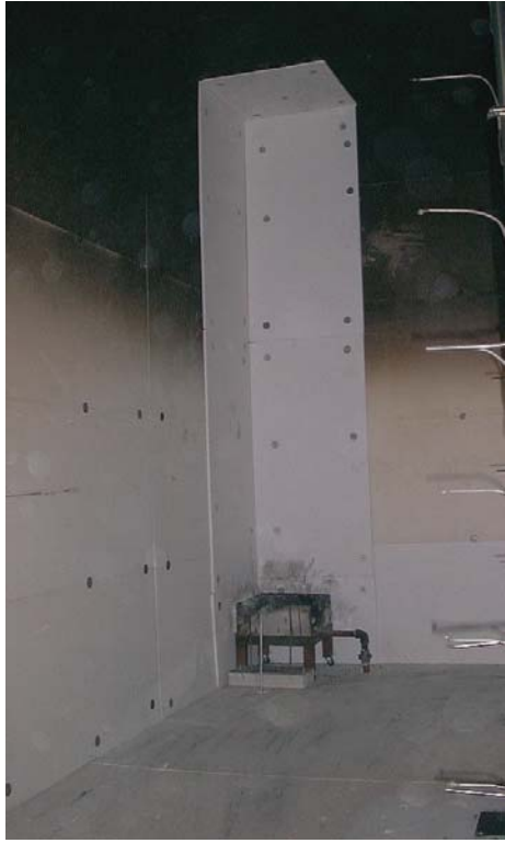
Figure 2.24. Burner in the corner location, with the second layer of insulation board attached.
