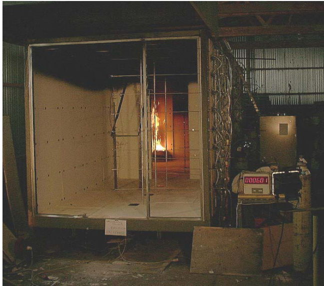
Figure 2.20. Front opening of compartment, unrestricted. The Burner can be seen in the corner location for this experiment.
