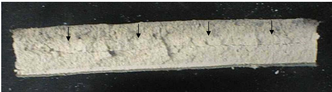
Figure 3.3 Examining the depth of calcination using the naked eye
