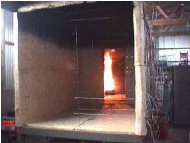
Figure 4.4 110 kW Corner Fire
