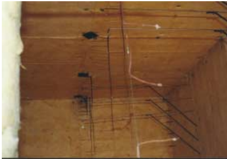
Figure 3.2 Field Thermocouple Trees in the Fire Room.
