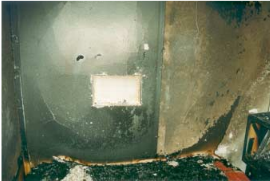
Figure 8-12: Different burn-off behaviour of paper exhibited by standard and fire rated plasterboard. (Note that GIB ® Fyreline is on the right of the picture and standard GIB ® board is on the left).
