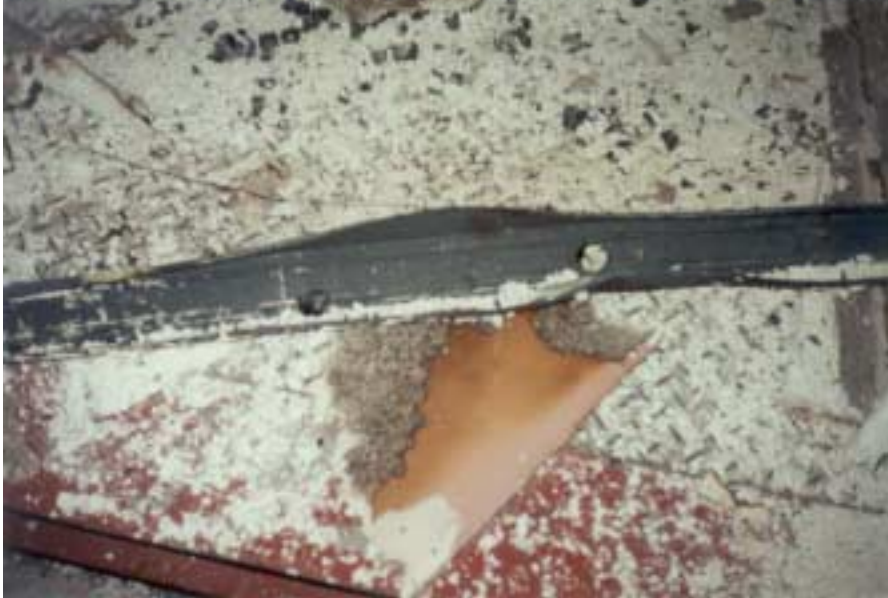
Figure 7-2: Buckling of steel stud from furnace test FP2881.
