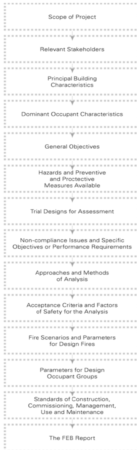
Figure 6.2: Areas for consideration prior to the formulation of a fire engineering brief
