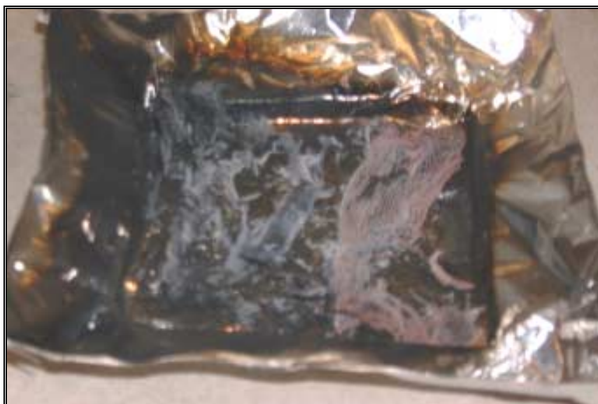
Figure 7-9: Photograph depicting the charred cellulose fibre strand that formed during the burning of composite K-34
