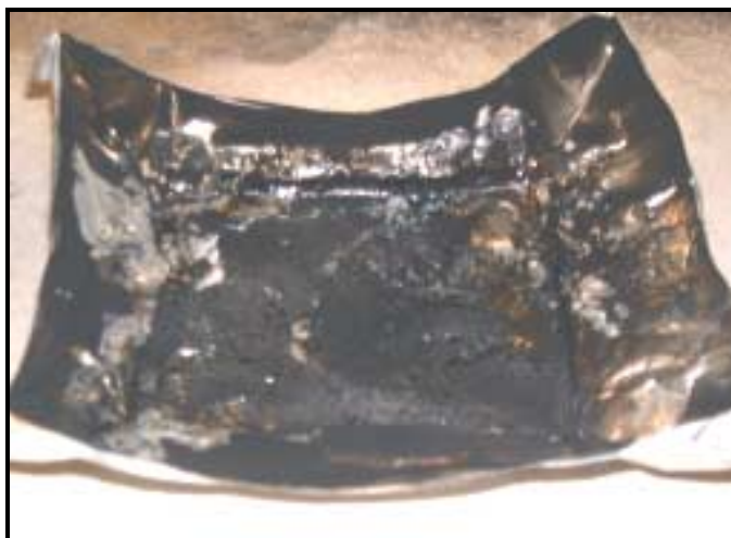
Figure 7-4: Photograph depicting the remnants of composite L-23 after burning.
